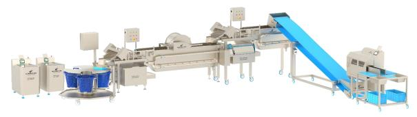
The ACBM in a vegetable processing line for cutting, washing and drying vegetables
